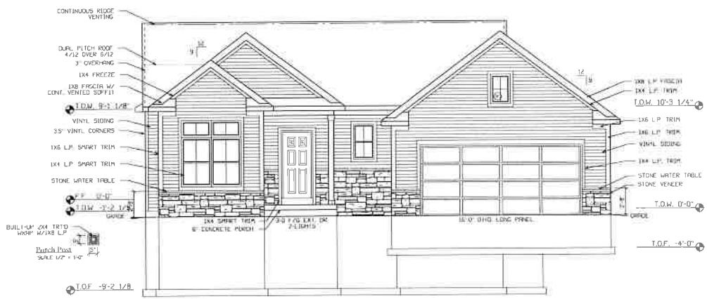
Front Elevation SCALE 1/4" = 1'-0"
